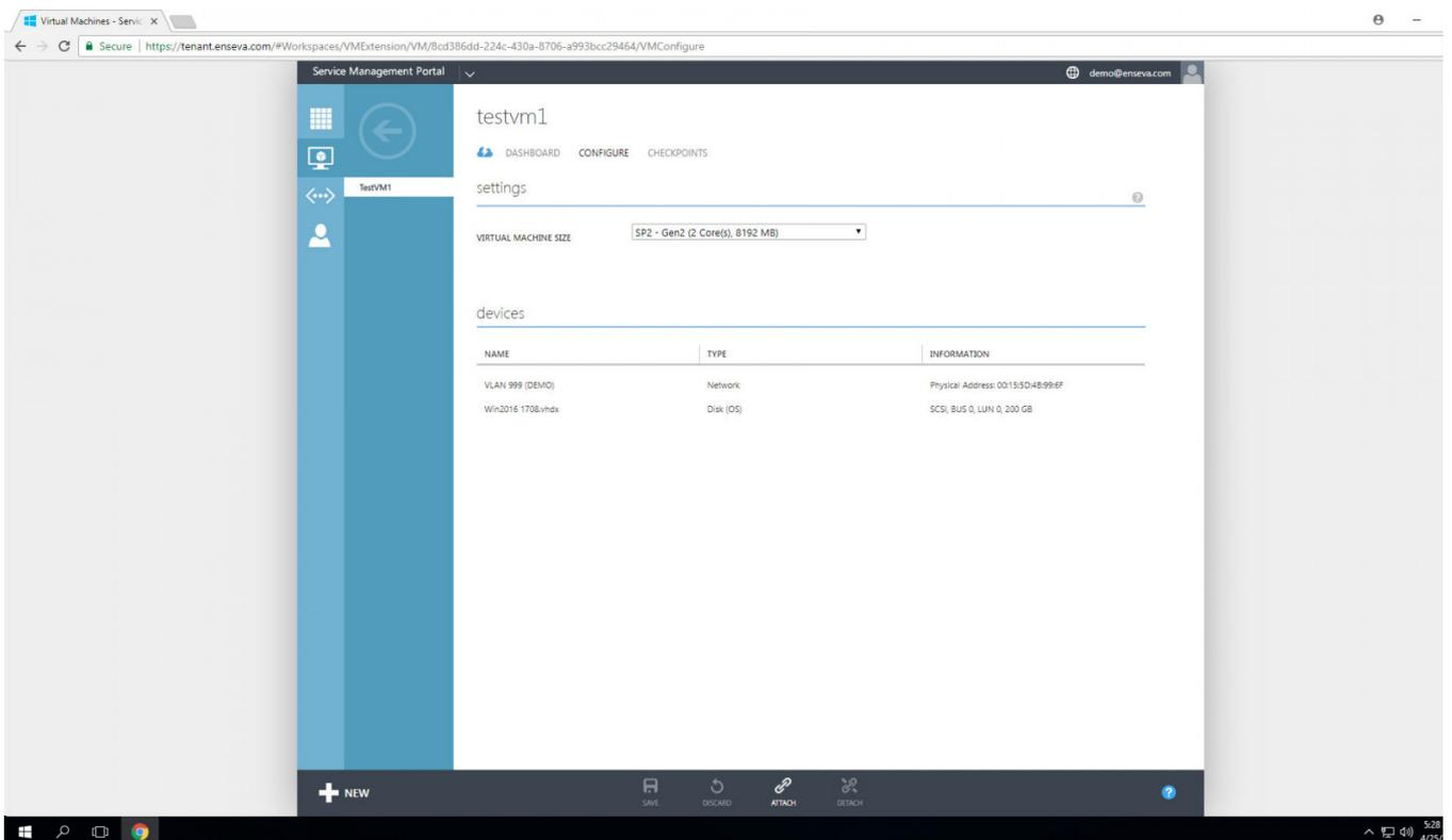
3. In the bottom menu, select the Attach button, followed by selecting Disk. This will launch the attach device wizard that will be utilized to add a new block storage device.
